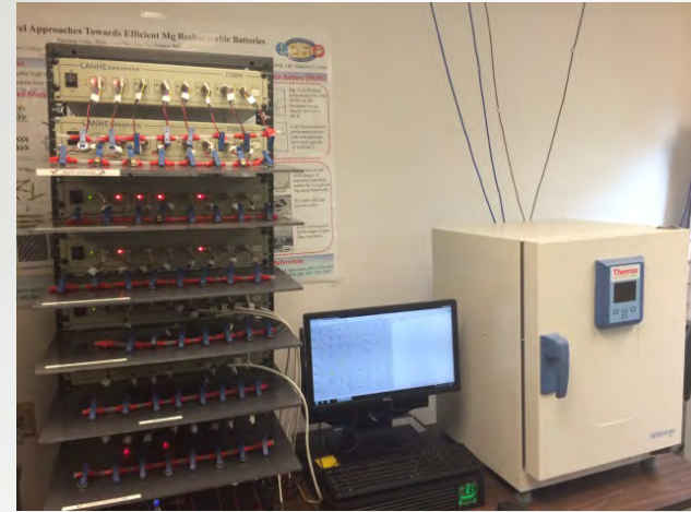
Battery testers with EIS (1MHz~0.01Hz)
