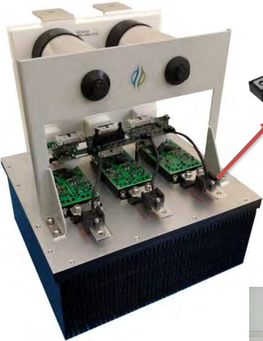
Agileswitch SiC Based 150 kW Inverter
