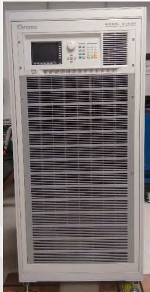
Regenerative Grid Simulator 0-300V, 10-100Hz, 30KVA
